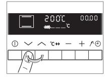
The oven function can be changed while the oven is working.
